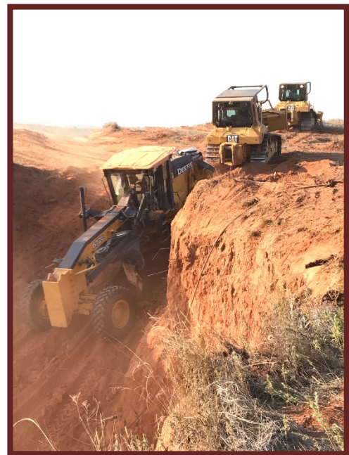
Two Type II dozers pulling motor grader from ravine
